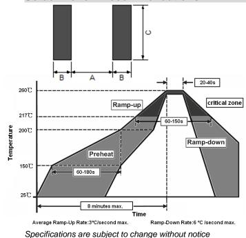
Devices are not designed to be wave soldered to the bottom
