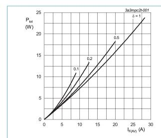
$I_{F(AV)} = I_{F(RMS)} \times \sqrt{\delta}$ V<sub>o</sub> = 0.667 V; R<sub>s</sub> = 0.0061 Ω
