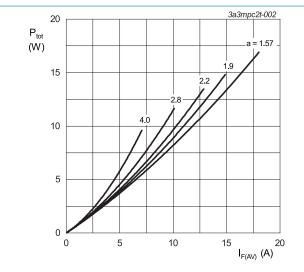
a = form factor =  $I_{F(RMS)} / I_{F(AV)}$  $V_o = 0.667 \text{ V}; R_s = 0.0061 \Omega$
