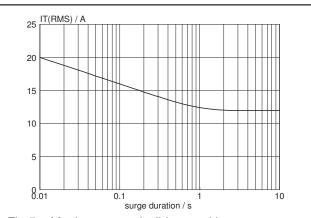
Fig.5. Maximum permissible repetitive rms on-state current  $I_{T(RIMS)}$ , versus surge duration, for sinusoidal currents, f = 50 Hz;  $T_{mb} \le 100$  °C.
