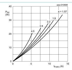
a = form factor =  $I_{F(RMS)}/I_{F(AV)}$  $V_o$  = 1.578;  $R_s$  = 0.027  $\Omega$
