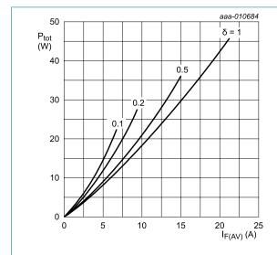
$V_o$  = 1.578;  $R_s$  = 0.027  $\Omega$ Fig. 1. Forward power dissipation as a function of average forward current; square waveform; maximum values
