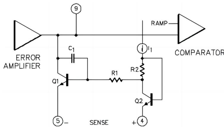
$$\text{C.L. Threshold} = V_{BE}(Q1) + I_1 \cdot R_2 - V_{BE}(Q2) = I_1 \cdot R_2 \\ \sim 200 \text{ mV}$$
