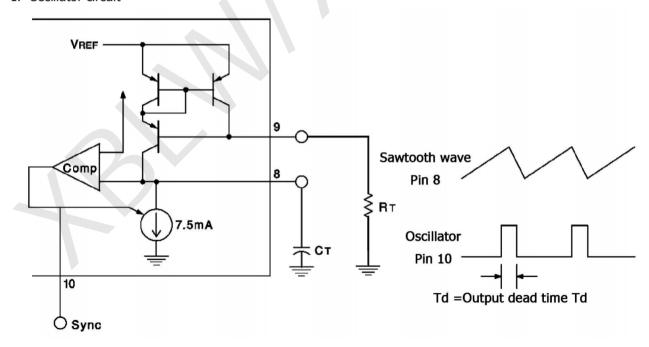
The output dead time is determined by the size of the external capacitance CT and is calculated as: TD =145\*CT [12/(12-3.6/RT)] where TD is in units of  $\mu$ s, C in units of  $\mu$ F, and RT in units of K $\Omega$  When the RT value is relatively large, TD ( $\mu$ s)=145\*CT( $\mu$ F); The oscillator frequency is approximately fT (KHz)=2.2/RT (K $\Omega$ )CT ( $\mu$ F).
