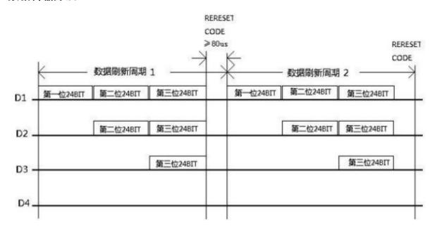
注: 其中 D1 为 MCU 端发送的数据,D2、D3、D4 为级联电路自动整形转发的数据 Note: D1 refers to the data sent by MCU, and D2, D3 and D4 refer to the data automatically shaped and forwarded by cascade circuit.
