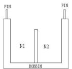
绕线结构表 Winding Structure Diagram
