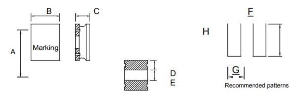
$A=2.5\pm0.3$   $B=2.0\pm0.3$  C=1.25 Max  $D=0.8\pm0.3$   $E=0.9\pm0.3$  F=0.6 G=1.1 H=2.0 marking: A
