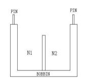
绕线结构表 Winding Structure Diagram
