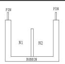
绕线结构表 Winding Structure Diagram
