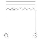
绕线结构表 Winding Structure Diagram
