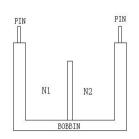
绕线结构表 Winding Structure Diagram
