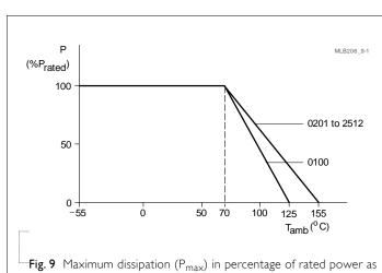
Fig. 9 Maximum dissipation ( $P_{max}$ ) in percentage of rated power as a function of the operating ambient temperature ( $T_{amb}$ )
