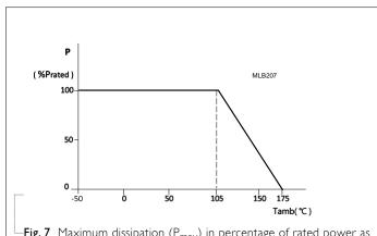
Fig. 7 Maximum dissipation ( $P_{max}$ ) in percentage of rated power as a function of the operating ambient temperature ( $T_{amb}$ )
