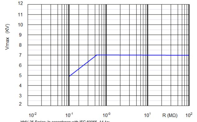
HHV-25 Series: In accordance with IEC 60065- 14.1a; 50 discharges from a 1 nF capacitor charged to Umax; 12 discharges/min
