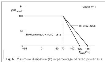
function of the operating ambient temperature (T<sub>amb</sub>)
