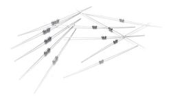
The MFO Series Metal Film Professional Resistors are manufactured using a vacuum sputtering system to deposit multiple layers of mixed metal alloys and passivative materials onto a carefully treated high grade ceramic substrate. After a helical groove has been cut in the resistive layer, tinned connecting leads of electrolytic copper are welded to the end-caps. The resistors are coated with layers of blue color lacquer.
