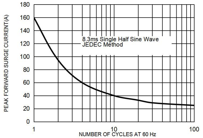
FIG. 2 MAXIMUM NON-REPETITIVE FORWARD SURGE CURRENT PER LEG
