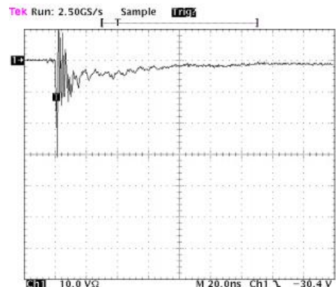
Figure4- ESD Clamping Voltage Screenshot Negative 8 kV Contact per IEC61000-4-2
