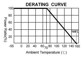
Power rating or current rating is in the case based on continuous full-load at ambient temperature of 70℃. For operation at ambient temperature in excess of 70°C, the load should be derated in accordance with figure of derating Curve.
