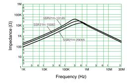
AC Line Filters - Common Mode SSR Coils, 21H Series, High Impedance Type
