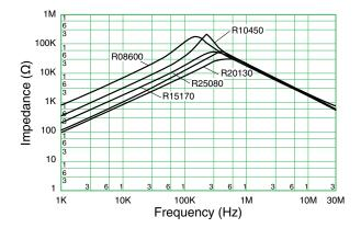
AC Line Filters - Common Mode SS Coils, B28V/H Series
