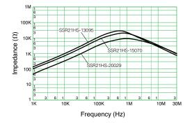
AC Line Filters - Common Mode SSR Coils, 21HS Series, Wide Range Impedance Series
