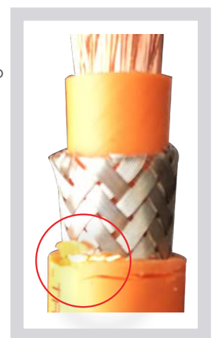
Figure 3. Example of damaged outer jacket
