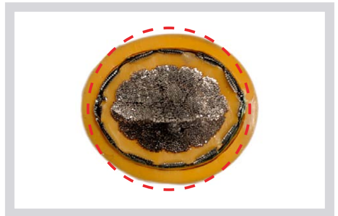
Figure 2. Example of “Footballing” in a 120 \text{ mm}^2 cable
