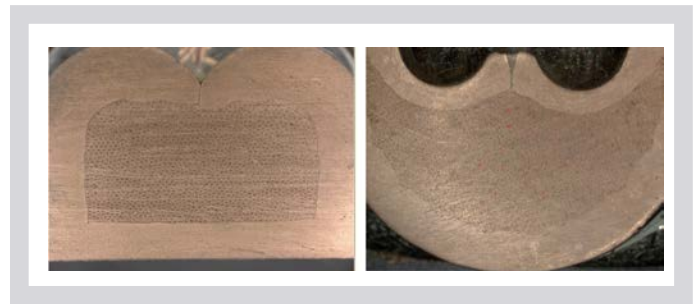
Figure 14. Examples of terminal cross-sections
