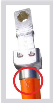
Figure 12. Example of loose braiding that could cause an electrical short
