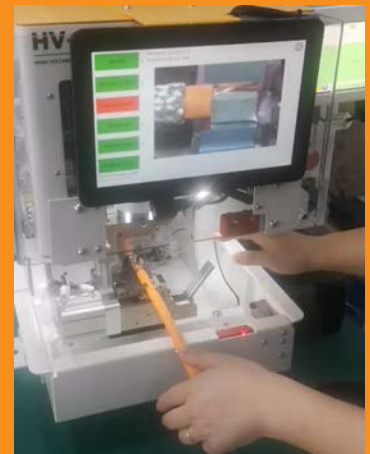
Figure 20. Example of advanced vision system validating a crimp
