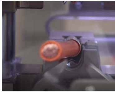
Figure 21. Example of an improperly bent wire
