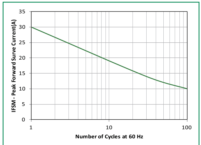
Figure 8 - Maximum Non-Repetitive Forward Surge Current Uni-Directional Only
