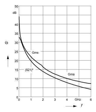
Power gain  $G_{\text{ma}}$ ,  $G_{\text{ms}}$  = f ( $V_{\text{CE}}$ )  $I_{\text{C}}$  = 20 mA
