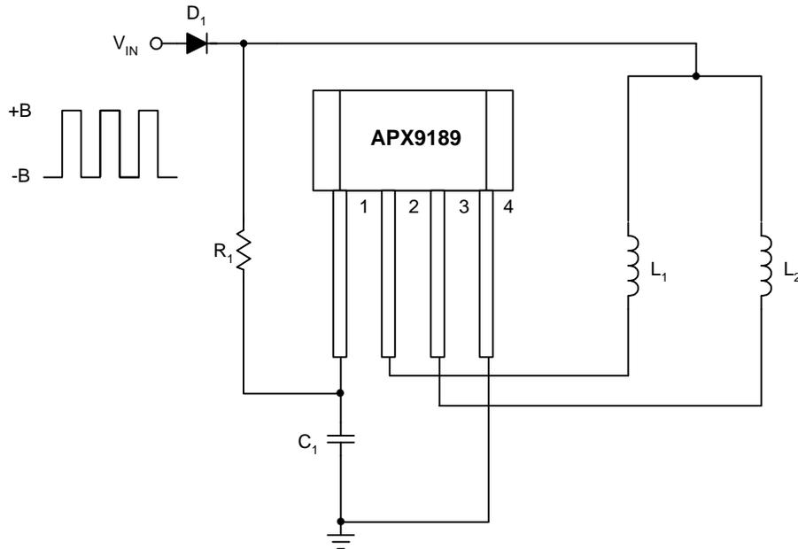
Notes:  $D_1$  is to protect circuit and coils when reverse power input.
