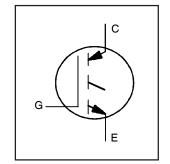
600 V  $I_{C(nom)} = 12A$   $V_{CE(on)} \text{ typ.} = 1.55V @$   $I_{C(nom)} @ 25^{\circ}C$ Motor Control IGBT
