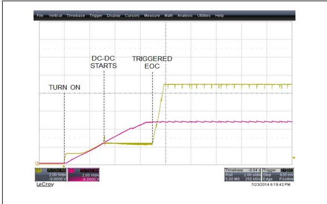
Figure 13. Buck-boost startup ( I_{IN} = 5\ \mu\text{A} )
