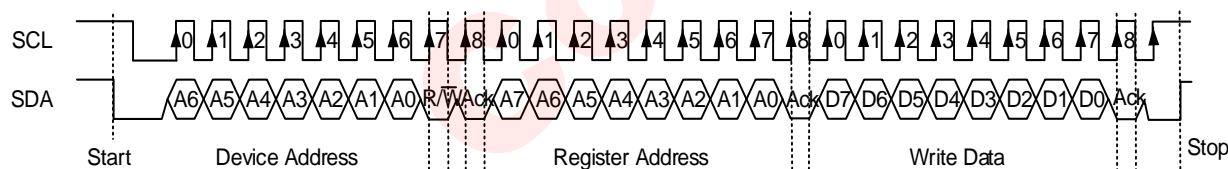
Figure 9 I 2 C Write Byte Cycle
