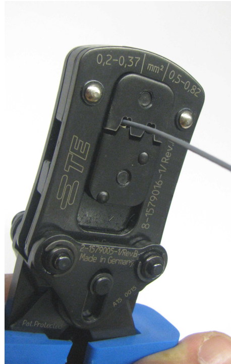
Picture 7: Squeezing handles and crimping
