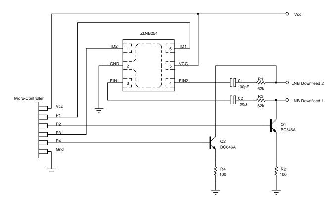
The above circuit shows the additional components that will be used in a typical ZLNB254 application operating at a Vcc of 5V and detecting 22kHz tones/tone bursts. The transistors Q1 and Q2 are not required for the ZLNB254 operation, they demonstrate how a DiSEqC 2.X (2 way communication) could be achieved.
