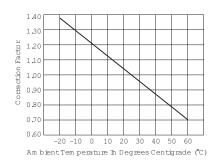
To use this chart: Read up from the ambient temperature to the curve, and across to find a correction factor. Multiply the breaker rating by the correction factor to determine the compensated rating. Calculate the overloads in terms of the compensated rating to use the published trip curve.
