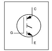
600 V  $I_{C(nom)} = 35 \text{A}$   $V_{CE(on)} \text{ typ.} = 1.6 \text{V} @$   $I_{C(nom)} @ 25 ^{\circ}\text{C}$  Motor Control IGBT Short Circuit Rated 150 mm Wafer
