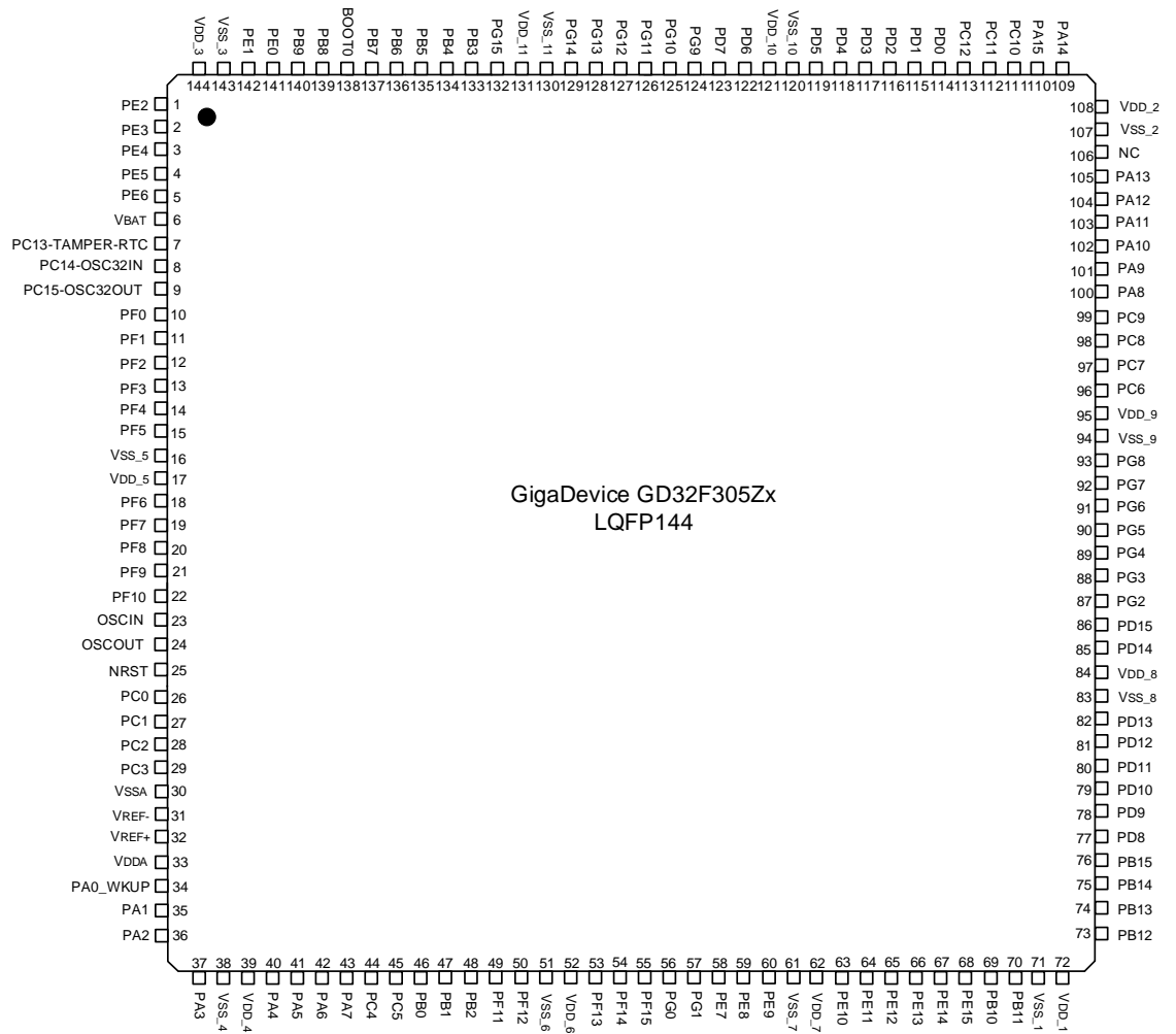
Figure 2-2. GD32F305Zx LQFP144 pinouts
