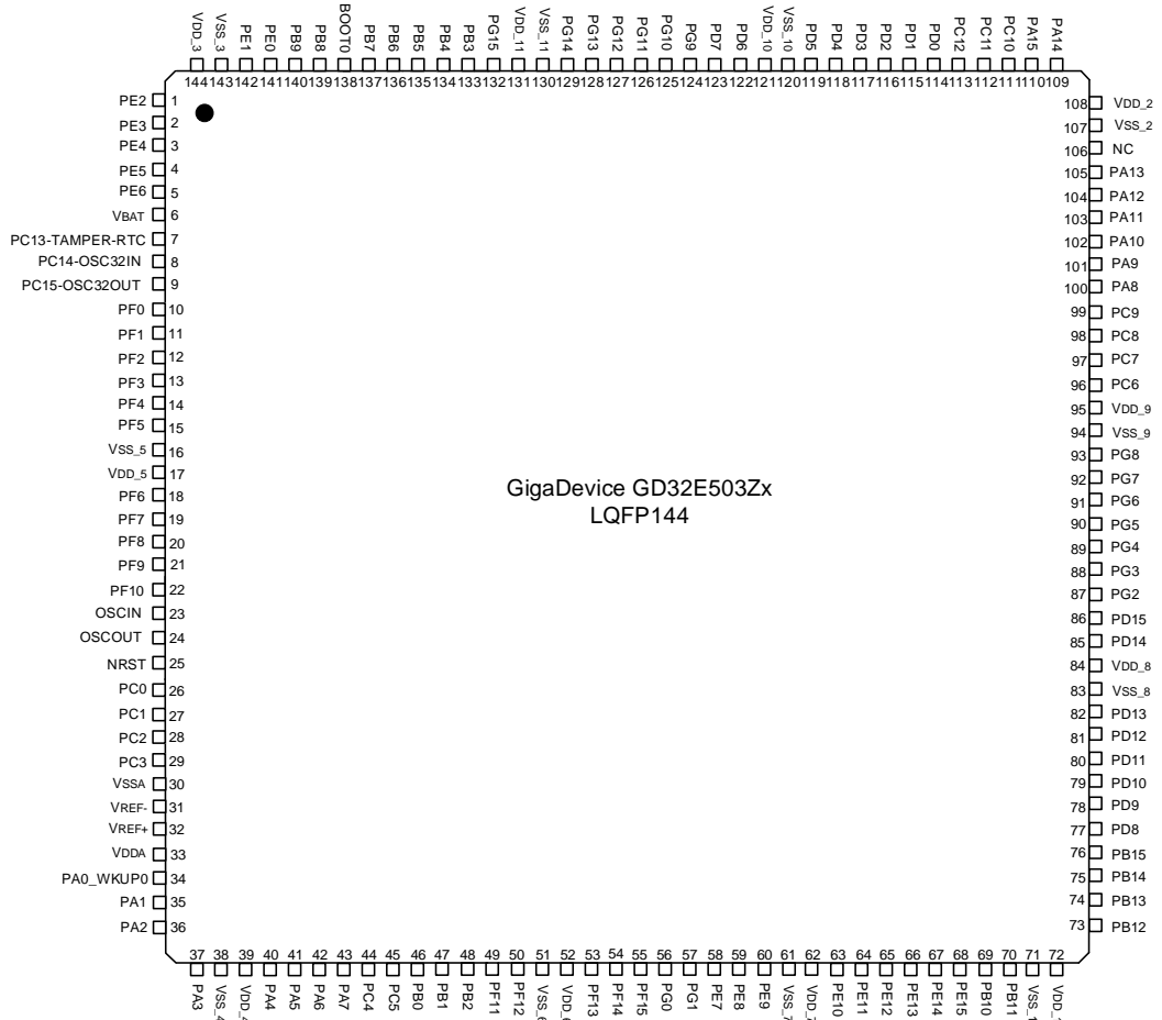
Figure 2-2. GD32E503Zx LQFP144 pinouts
