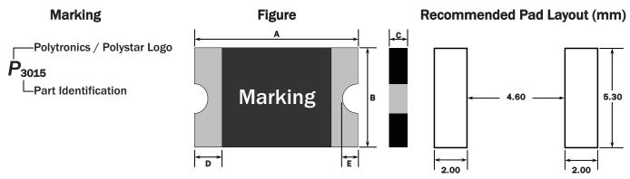
Note: Polystar is Polytronics's manufacturing site in China. The Polystar ID marking shall appear on smallest package.
