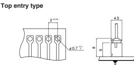
Note: 1. Tolerances are non-cumulative: ±0.05mm for all centers. 2. Hole dimensions differ according to the kind of PC board and piercing method. If PC boards made of hard material are used, the hole dimensions should be larger. The dimensions above should serve as a guideline. Contact JST for details.
