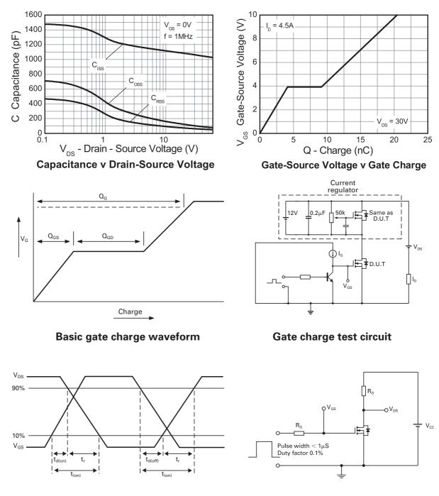
Switching time waveforms
