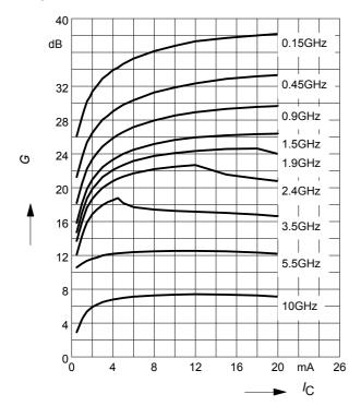
**Power gain**  $G_{ma}$ ,  $G_{ms}$ ,  $|S_{21}|^2 = f(f)$  $V_{CE} = 3 \text{ V}$ ,  $I_C = 5 \text{ mA}$
