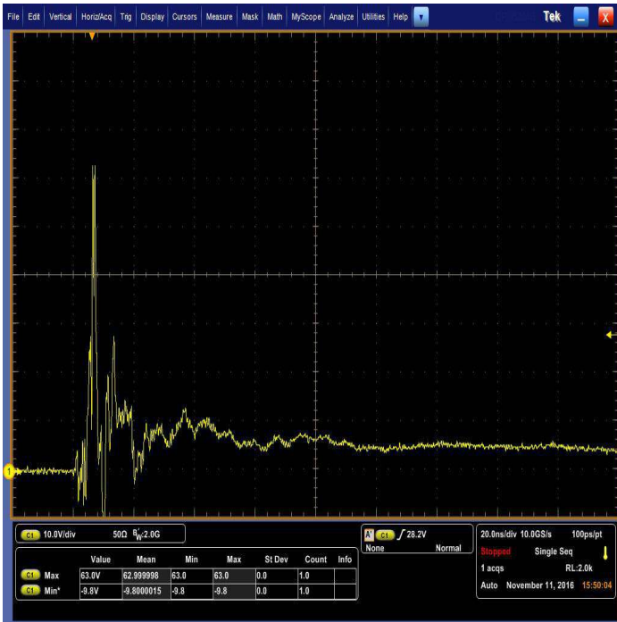
Figure 3. Positive 8kV contact per IEC 61000-4-2
