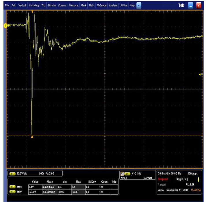
Fig 4. Negative 8kV contact per IEC 61000-4-2
