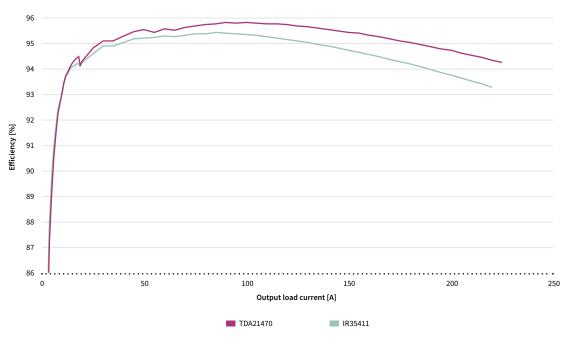
Efficiency levels at  $f_{sw}$  = 500 kHz,  $V_{in}$  = 12 V,  $V_{out}$  = 1.82 V, five-phase measurement
