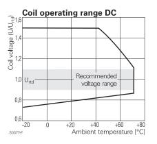
Datasheets and product specification according to IEC 61810-1 and to be used only together with the 'Definitions' section.
