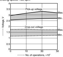
4. Electrical life (1A 30V DC resistive load) Tested sample: AGN2004H, 6 pcs. Operating speed: 20 cpm Change of pick-up and drop-out voltage
