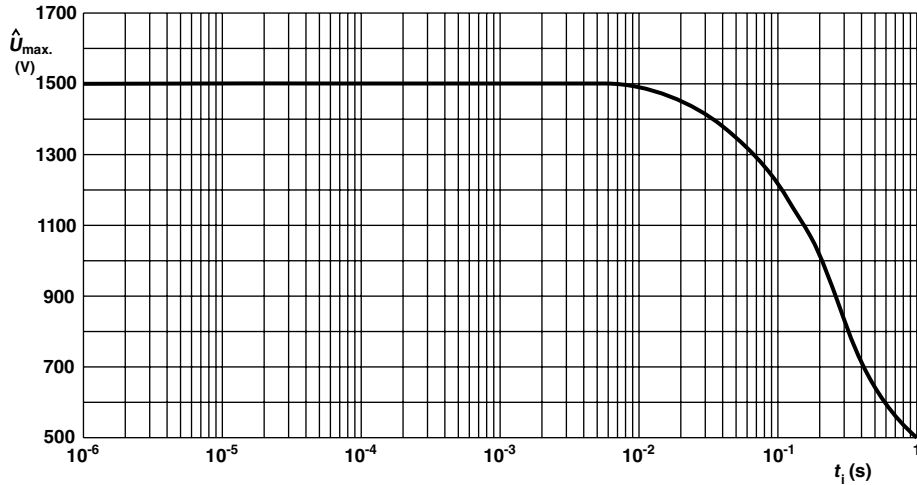
PR02 Pulse on a regular basis; maximum permissible peak pulse voltage ( \hat{U}_{max.} ) as a function of pulse duration ( t_i )
