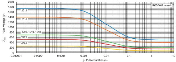
Maximum pulse voltage, single and continuous pulses; applicable if  $\hat{P} = \hat{P}_{\text{max}}$ ; for permissible resistance change equivalent to 8000 h operation
