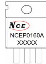
Marking and pin assignment
