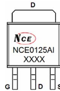
Marking and pin assignment
