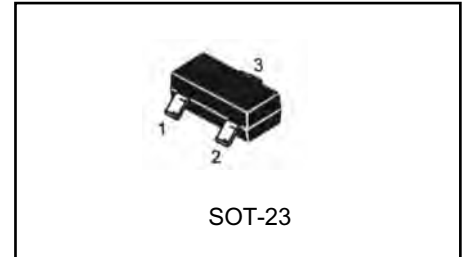
SOT-23 1: Ref; 2: Cathode; 3: Anode
